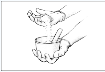
Figure 4 Stir in small quantities of filler until the desired consistency is reached.
