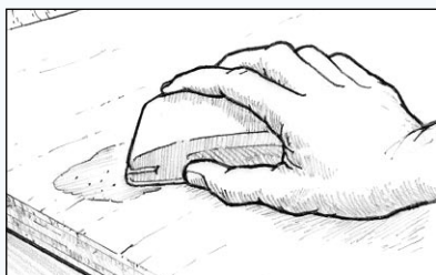
Figure 23 Sand cured fairing compound to desired contour.
