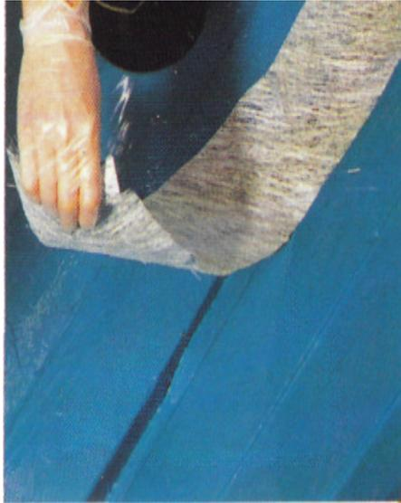
5) Lay down a strip of chopped strand mat along the keel line. Stipple it into the wet resin with a brush. Remember-do NOT "paint" to and fro. A resin applicator roller can be used instead of a brush. Put down
