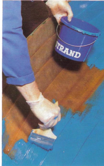
4) Mix catalyst into a working quantity of the pigmented lay up resin (Resin A). Paint the Resin A over the gelcoat.
