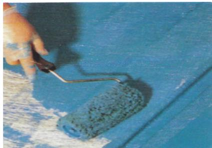
more glassfibre until the mould surface is covered. Prevent the resin on the brushes and tools from beginning to solidify -leave them to soak in Brush Cleaner whilst you continue working with fresh brushes.
