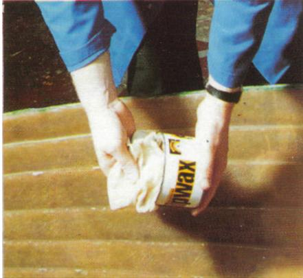
before buffing it thoroughly then applying the next. The final coat should be covered with Wax Release Agent. Leave to dry for about 15 minutes before laminating.
