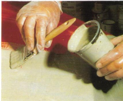
5) Add catalyst to lay-up resin (Resin A). Paint the Resin A over the gelcoat.
