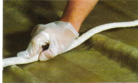
Laminate over the paper rope to create strengthening ribs.
