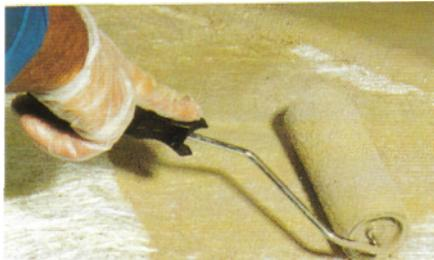
7) Make sure the glassfibre is thoroughly impregnated with resin ("wetted out"), then use a metal laminating roller to consolidate the layer. As you continue
